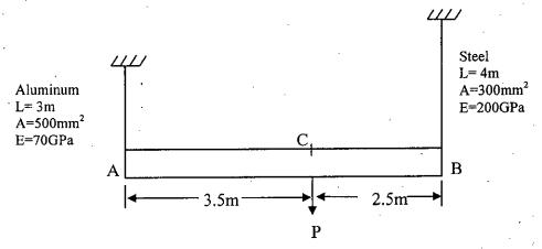
A rigid bar of negligible weight is supported as shown in figure. If W=80 kN, compute 2(a) the temperature change that will cause the stress in the steel rod to be 55MPa. Assume the coefficients of linear expansion are 11.7  $\mu$  m/(m°c) for steel and 18.9  $\mu$  m/(m°c) for bronze.
