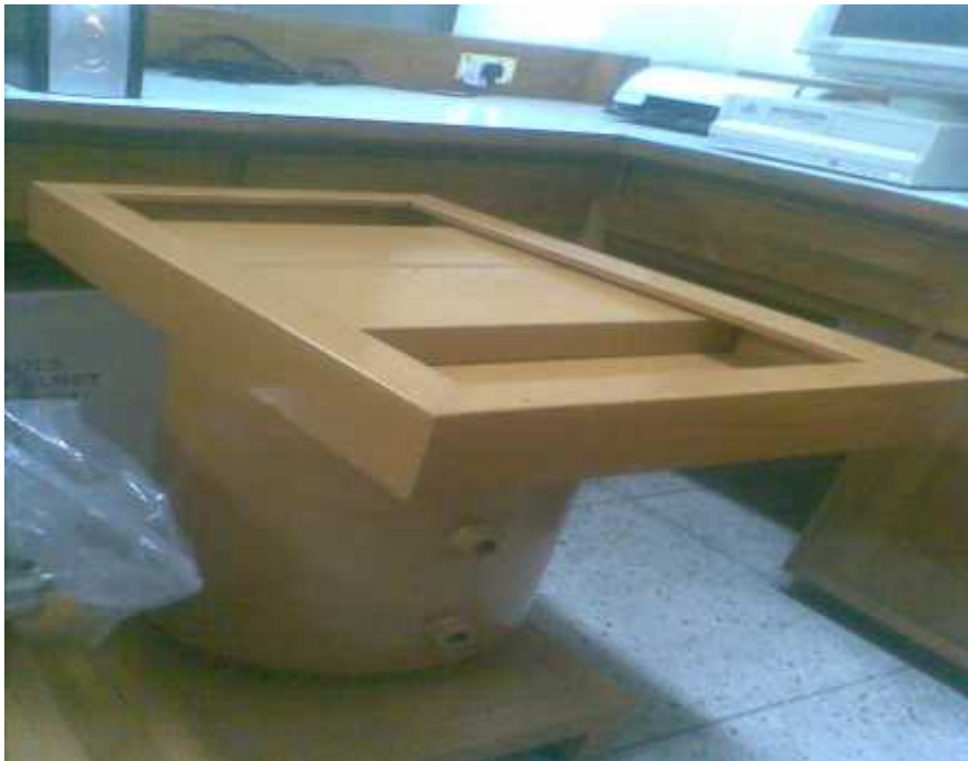
Fig 3.9: Photograph of the Shielding Arrangement of the Detector
