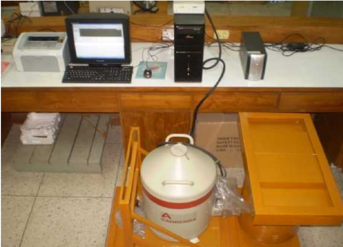
Fig 3.5: A complete setup of \gamma -counting system (HPGe Detector with 20% relative efficiency).
