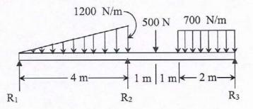
7(b) Determine the support moments and reactions for the beam as shown in figure.
