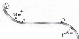
3(b) 2.5 kg collar is attached to a spring and slides without friction in a vertical frame along the curved rod ABC. The spring is undeformed when the collar is at C and its constant is 600 N/m. If the collar is released at A with no initial velocity, determine its velocity (i) as it passes through B, and (ii) as it reaches at C.
