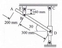
6(b) End A of rod AB has velocity of 2.5 m/sec and an acceleration of 1.5 m/sec<sup>2</sup> both 18 directed to right. Determine (i) the angular acceleration of rod AB, and (ii) the acceleration of the midpoint of rod AB.
